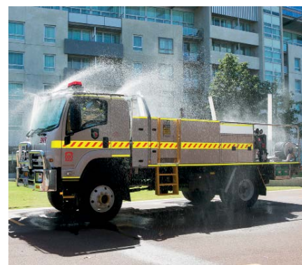
External water deluge system in action, photo courtesy of DFES
